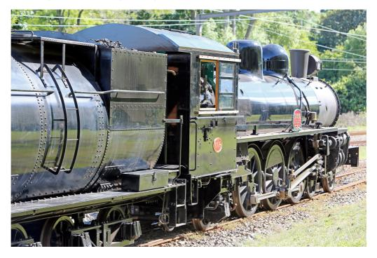
The reassembly of our Society's leased locomotive Ab 608 continues to progress at Steam Inc., Paekakariki. The tender is now on its own bogies again and is coupled to the engine. At the time this photograph was taken one name plate had been fitted. The other was still being re-painted., November., 2013.
