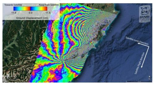
This image is an interferogram, produced using data from a Japanese Space Agency satellite. Each set of rainbow-coloured contours represent 11.5cm of movement. Where the coloured contours are closest together is where the largest changes in land motion are occurring.
