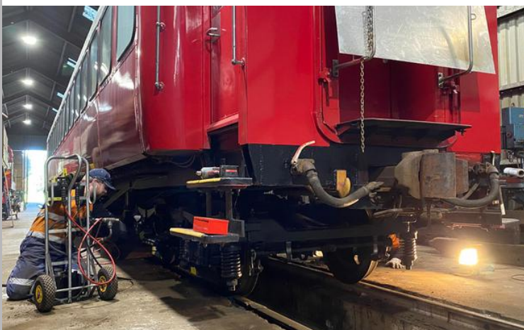
Left: Jack operates the jacks to lower the car onto the bogie. Right: Team Garratt, John and Russell contemplate the next job.
