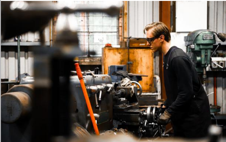
Left: The apprentice churning out brake pins for A1975's bogie overhaul. Right: Peter and Dave survey the bogie for cracks and defects
