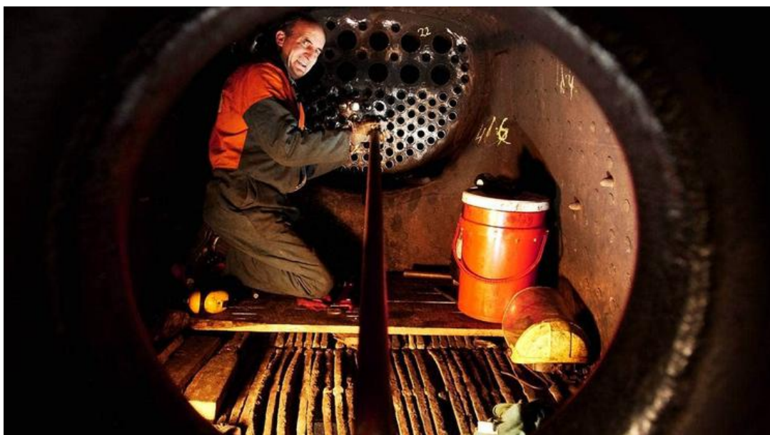
Bill Noble puts in the first of 110 tubes in AB699's boiler in 2005 - John Bisset
