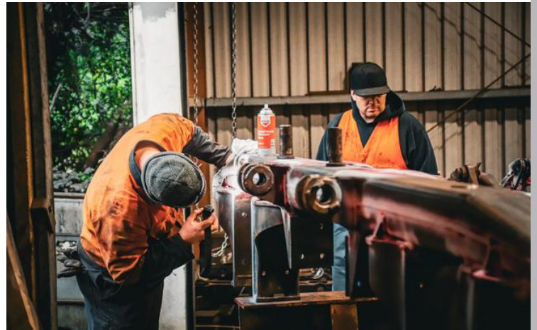
Left: The apprentice churning out brake pins for A1975's bogie overhaul. Right: Peter and Dave survey the bogie for cracks and defects
