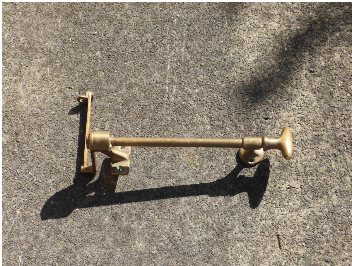
An example of a top light opener we will need to make from new, it has 7 separate parts
