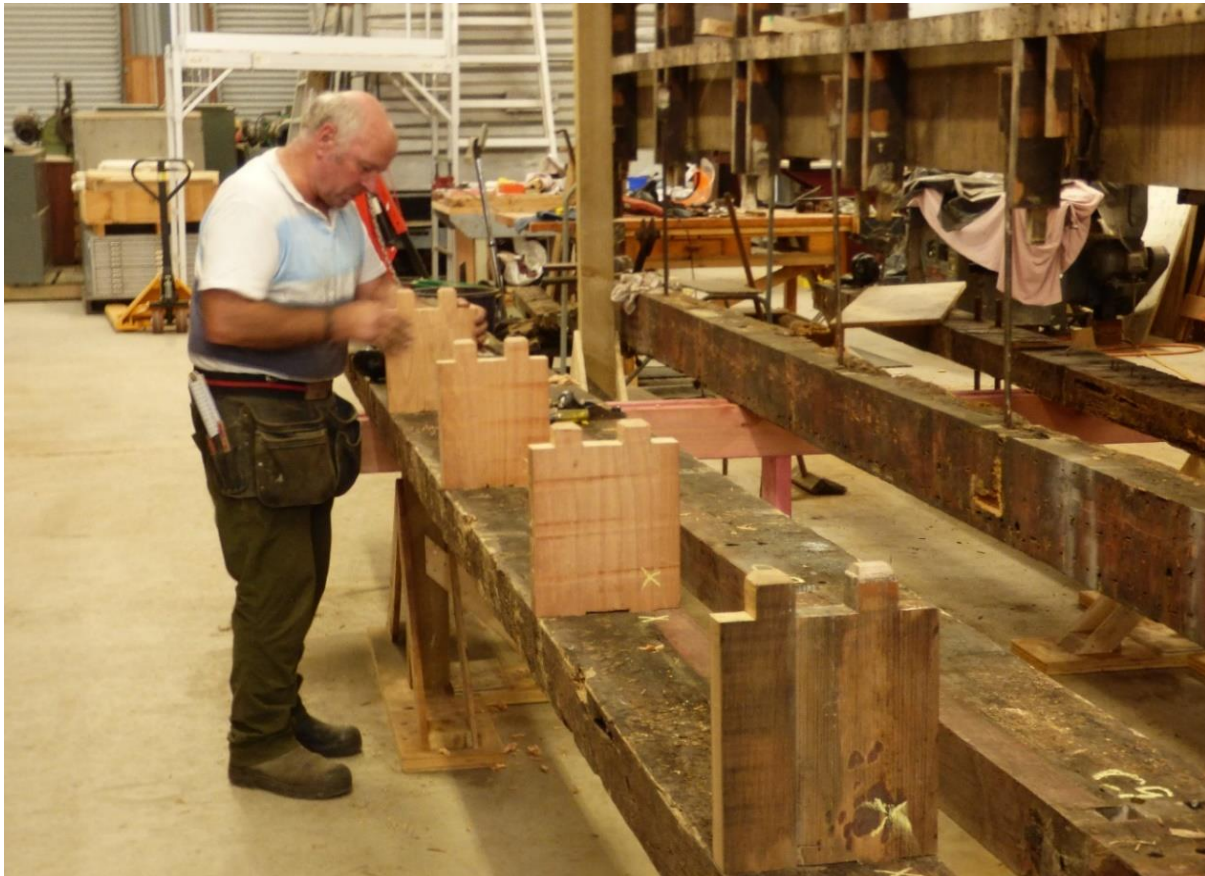
Kevin Cottle working on a trial re-assembly of pieces for the central spine beam of WMR 52.
